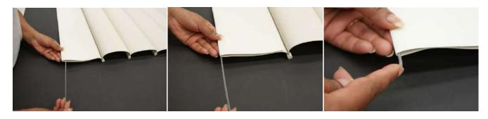
2. Place the Base Rail applicator onto the end of the base rail
