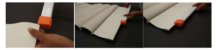
4. While continuing to pinch the fabric, proceed to slide the Base Rail Profile along the width of the fabric until the outer end is level with the edge of the skin. NOTE – be sure to <u>Push</u> the Base Rail Profile <u>Do Not</u> Pull the Base Rail Profile using the Base Rail Applicator
