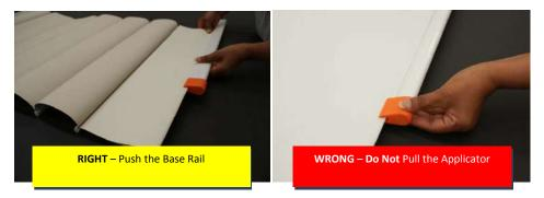
5 Continue to push the Base Rail Profile until you have reached the opposite side of the blind & remove the applicator
