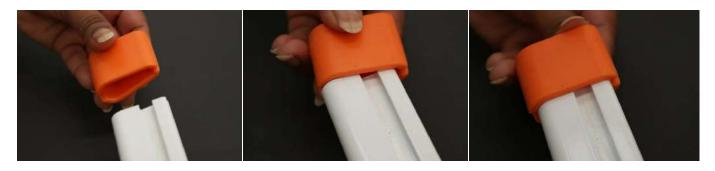
3. Pinch the fabric and slide the Base Rail Applicator onto the exposed Romatech Spline and onto the fabric.
