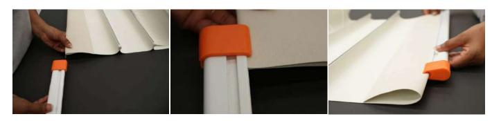
While continuing to pinch the fabric, proceed to slide the Base Rail Profile along the width of the fabric until the outer end is level with the edge of the skin. NOTE – be sure to <u>Push</u> the Base Rail Profile <u>Do Not</u> Pull the Base Rail Profile using the Base Rail Applicator.
