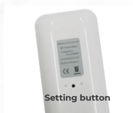
**2.** Press the setting button on the remote until the motor jogs.
