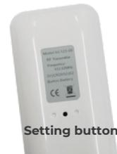
2. Press the setting button on the remote until the motor jogs.
