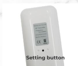
**4.** Press the setting button on the remote until the motor jogs.
